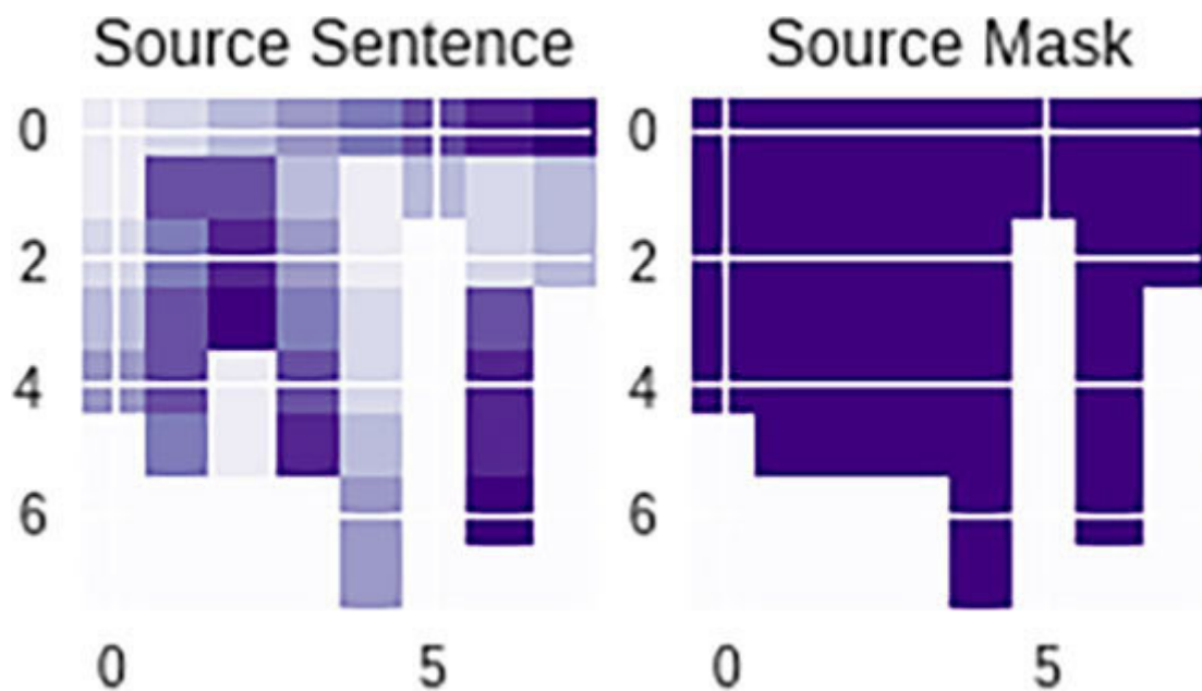
Figure 6.13: Masking applied to source sentences in the transformer.
