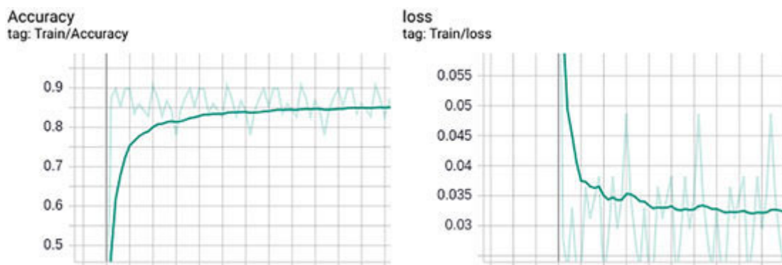
Figure 7.20: Decrease in loss and increase in accuracy on train data when model trains NER task taking character-level feature.
